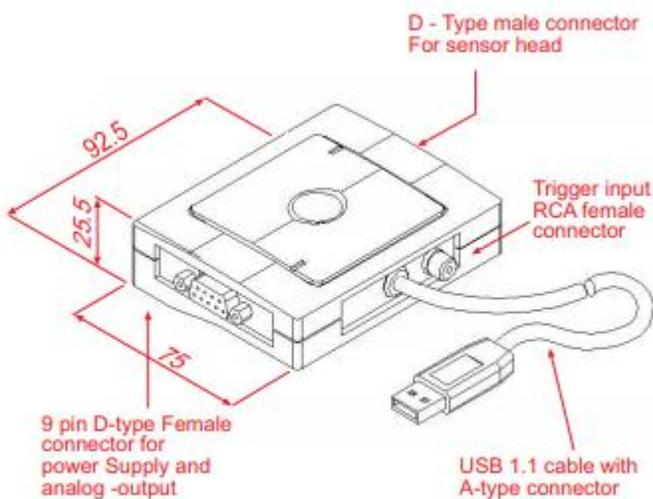
Dimensions are in millimeters
