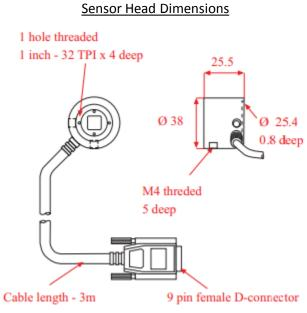
Dimensions are in millimeters
