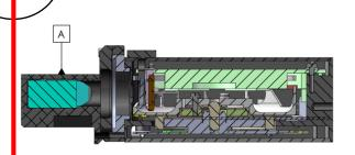
Optical distance from Input plane A to Detector Plane: 41±0.3
