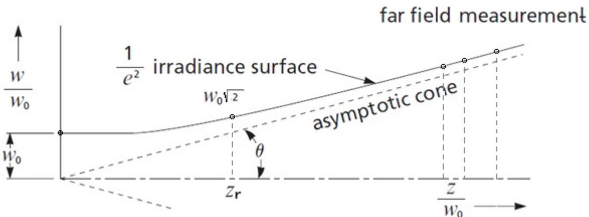
Figure 1 Describes the laser beam propagation along Z axis and possible locations for beam profile measurement
