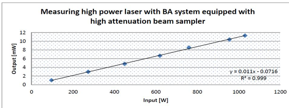
Figure 7 Test sampling ratio as a function of power for a typical beam sampler
