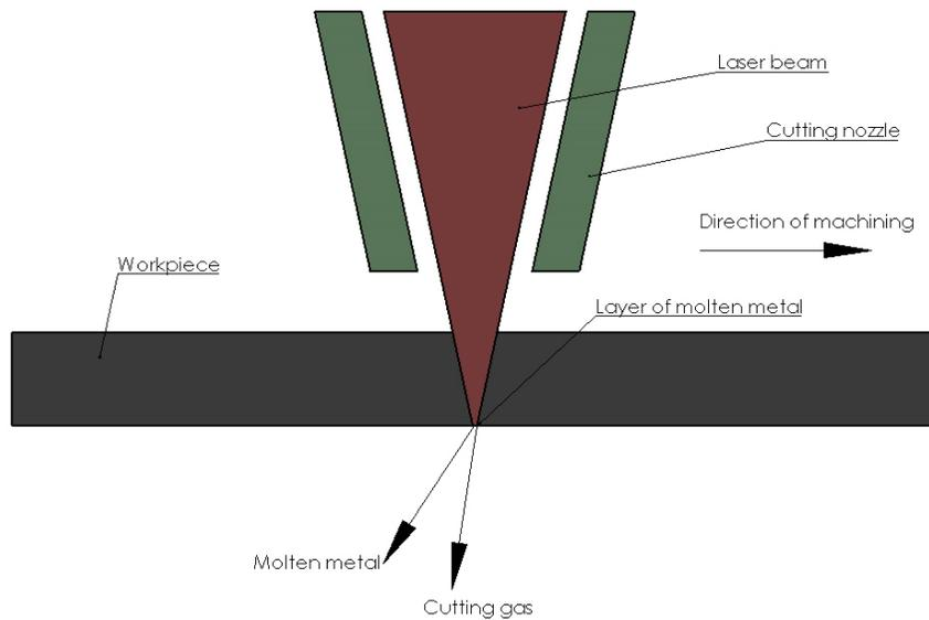
Figure 5 Describes the laser cutting procedure.
