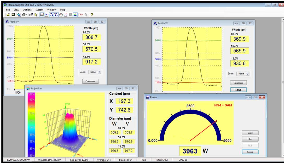
Figure 11 High Power laser beam profiler screens
