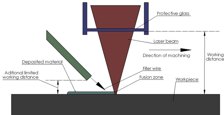
Figure 4 Describes a typical deposition welding head.
