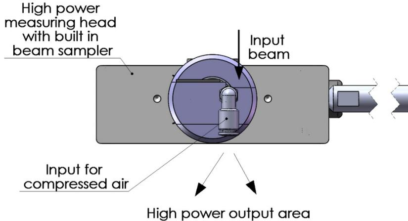
Figure 6 A multiple knife-edge measuring head equipped with custom beam sampler and compressed air cooling.
