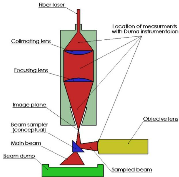
Figure 9 Schematic layout showing a typical measurement for a small work distance laser
